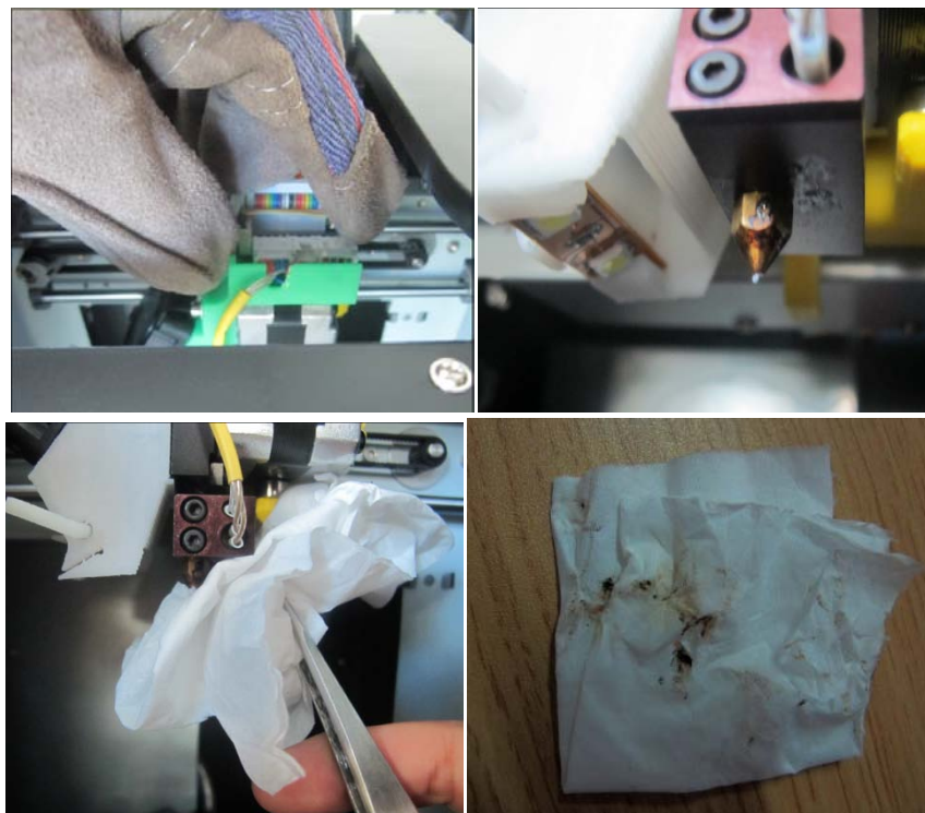
Figure 6-5 Nettoyage de la buse
