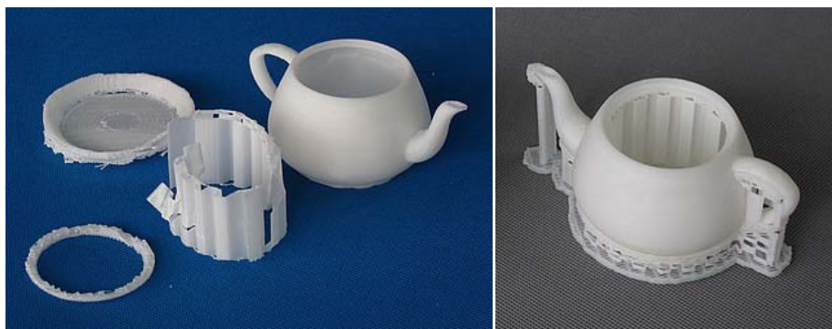
Figure 5-2 Structure de support
