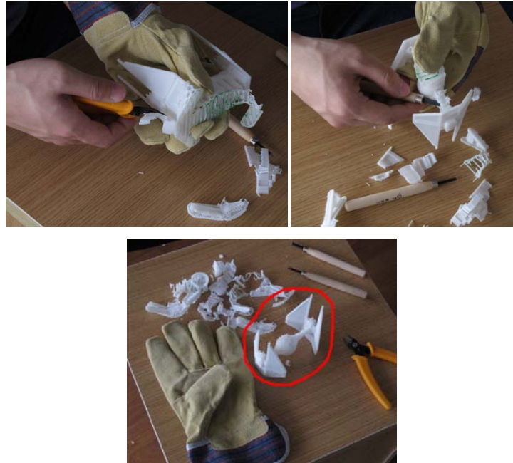
Figure 5-3 Retrait de la structure de support
